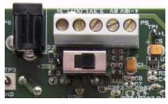
Figure 3: SmartRF04EB Power switch, power on.
